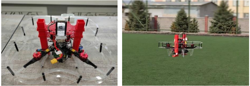
Figure 6. (left) Seed Sowing Drone, (right) Testing the drone.
